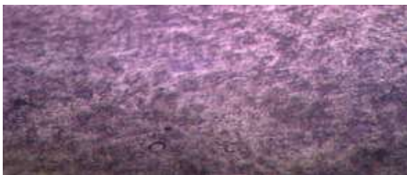
Fig3.4. Image of ALUMINIUM 6063 ALLOY +1 wt% \gamma - Al_2O_3 , ( magnification factor 100X)
