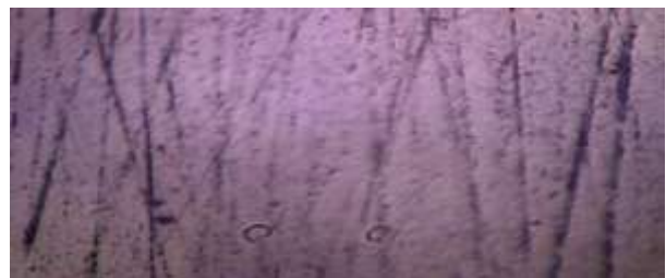
Fig3.4. Image of ALUMINIUM 6063 ALLOY +1 wt% \gamma - Al_2O_3 , ( magnification factor 100X)
