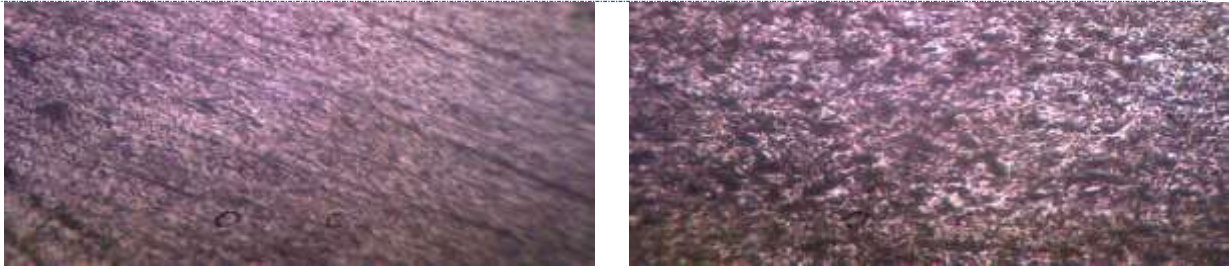
Fig3.6. Image of ALUMINIUM 6063 ALLOY + 3 wt% \gamma - Al_2O_3 , ( magnification factor 100X)
