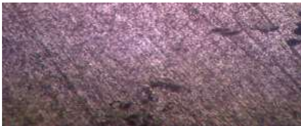
Fig3.3. Image of ALUMINIUM 6063 ALLOY +0.5 wt% \gamma - Al_2O_3 , ( magnification factor 100X)
