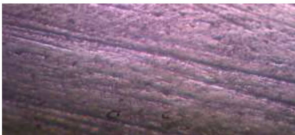
Fig3.5. Image of ALUMINIUM 6063 ALLOY +2 wt% \gamma - Al_2O_3 , ( magnification factor 100X)
